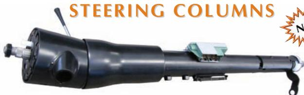
These steering columns are remanufactured original units re-painted black. New ignition switches (1969-74) and turn signal switches are installed. Steering wheel and components are not included.
