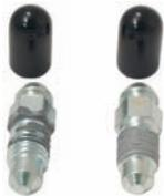
Bleeding your brakes has never been easier. Revolutionary Russell speed bleeder replaces the original bleeder screw in your wheel cylinder or caliper with a spring-loaded one-way ball and check valve design. The uniqueness of the stainless steel check ball is that it opens to allow fluid and air out, then closes automatically between pumps preventing air from reentering. It is now a one-person job with the speed bleeder.
