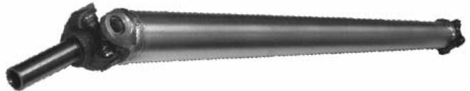
These driveshafts are constructed with 3" steel tubing with .083" wall thickness. They do not have the same step-tube design as original. Included are heavy-duty non-greaseable U-joints with a double-lip seal design for optimum grease retention. All driveshafts are shipped directly from the manufacturer. Driveshafts are bare steel and will need to be painted to prevent rust.
