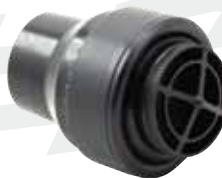
Round Aircraft Style Aluminum Vents, adjustable direction and rotating center for variable airflow control. 3" O.D. (Requires 2-3/4" hole).
