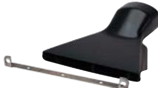
Defrost Outlet Kit 32-2455 ..... Defrost Outlet Can be trimmed shorter or angled Use Grill 32-2456 or 45-3256
