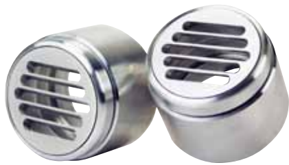
45-1610 ..... for 2" or 2-1/2" Duct Hose Round Aluminum Vents, Satin finish with rotating center for control of air flow direction. 2-3/8" O.D. (2-1/8" hole).
